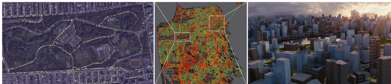
Fig. 1. 2D animation (left) and visualization (center) of reconstructed traffic in virtual San Francisco with 3D vehicle flows (right) using our method.
