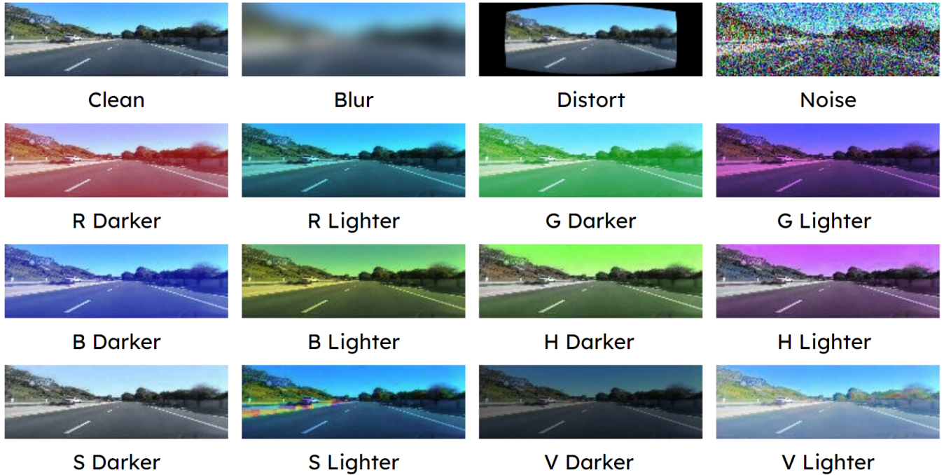
Fig. 3: Sample images used during training within the SullyChen [14] dataset. The clean image and its perturbed variants using all base perturbations are shown. The intensity level of the images is 0.5, half of the max intensity.
